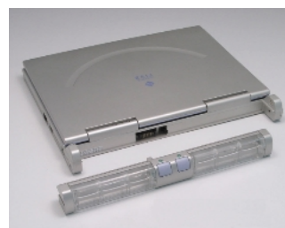
The long, slim part is the fuel cell.
